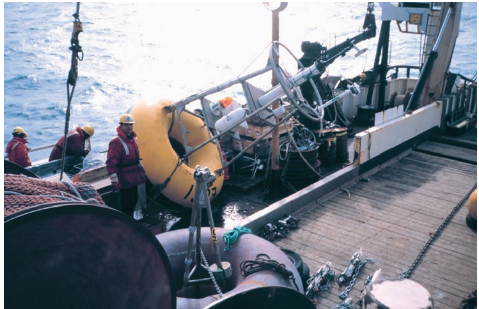
Figure 3.17 Once this weather buoy is deployed and is anchored in the ocean, it will collect data about the atmosphere and ocean. Data from this buoy, as well as others, are transmitted to a central location where they are analyzed and interpreted by computers.
