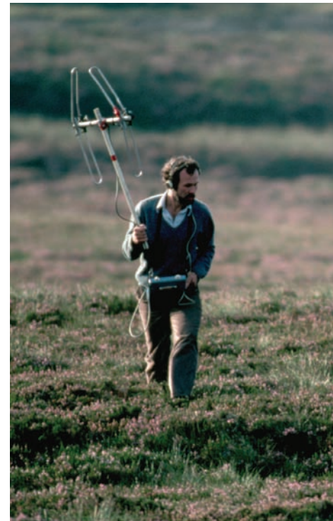
Figure 3.19 This researcher is holding an antenna to detect radio signals transmitted from an animal with a radio collar.
