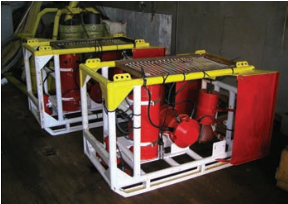
Figure 2.12 Deep sea cameras such as the NEPTUNE can reach ocean depths of 6 km.
