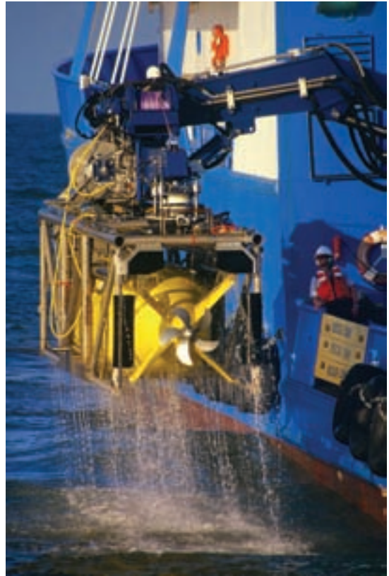
Figure 2.11 Remotely-operated vehicles are controlled by people from the surface. They can collect data, pictures, and objects.
