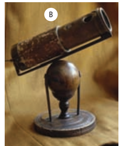
Figure 6.27 (A) Galileo used lenses to build simple telescopes that he used to make discoveries about the Universe. (B) Isaac Newton improved on Galileo's design by using a mirror to collect and begin to focus the light from the stars. This is now known as a reflecting telescope.
