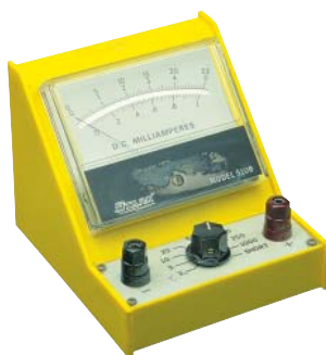
B. Analogue meters have a needle pointing to different scales.
