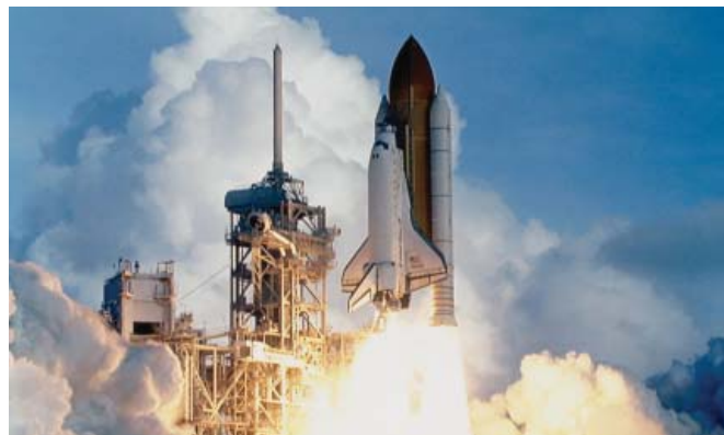
Figure 3.13 Combustion occurs when liquid hydrogen fuel reacts chemically with liquid oxygen within the shuttle's rockets. Light, heat, and sound are produced, along with a stream of hot gases that expand and propel the shuttle upwards.
