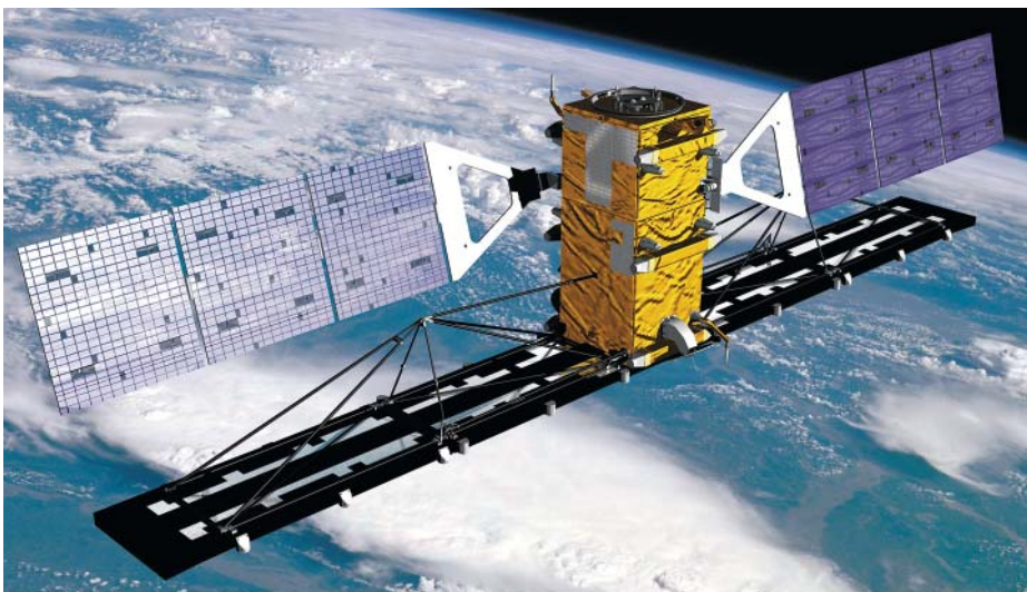
Figure 11.31 One of the Canadian Space Agency's first remote sensing satellites was RADARSAT 1 . RADARSAT 2 , shown to the left, is the newer version, and is used for geological mapping, forest mapping, iceberg detection, and marine surveillance.
