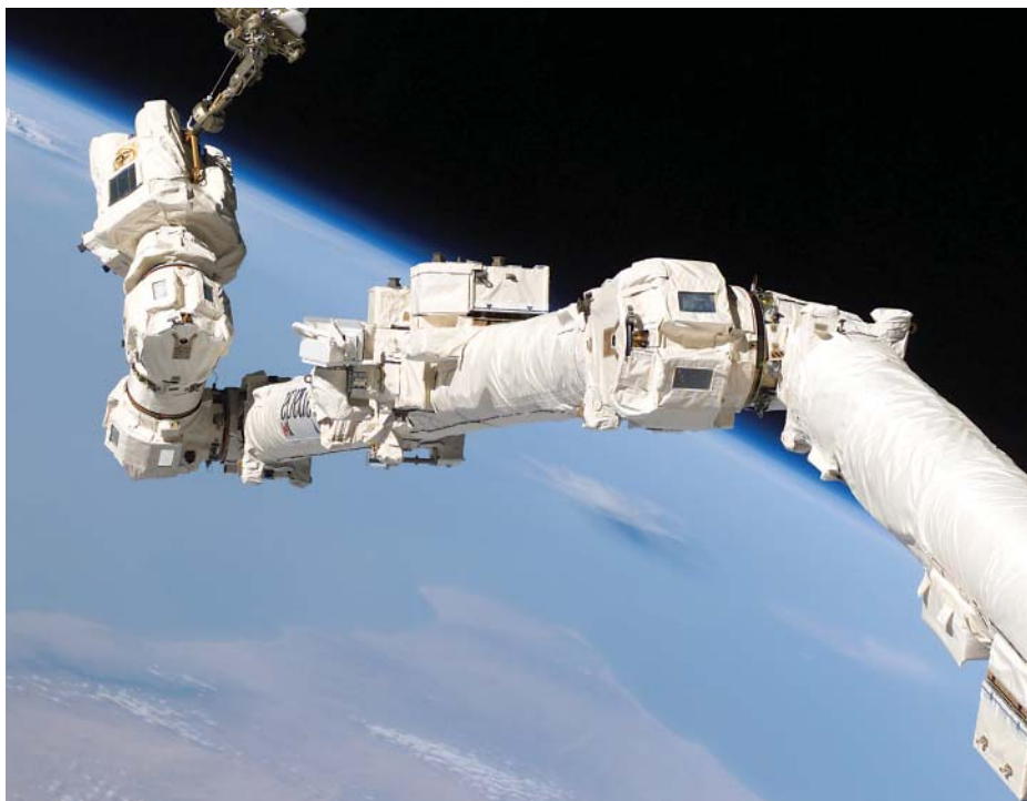
Figure 11.27 Canadarm 2 is used to move large payloads, dock the shuttle, and assist astronauts with repair and assembly duties.
