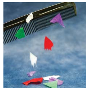
Figure 7.9 Even though the comb is not touching the paper on the table, the paper is attracted to the charged comb.
