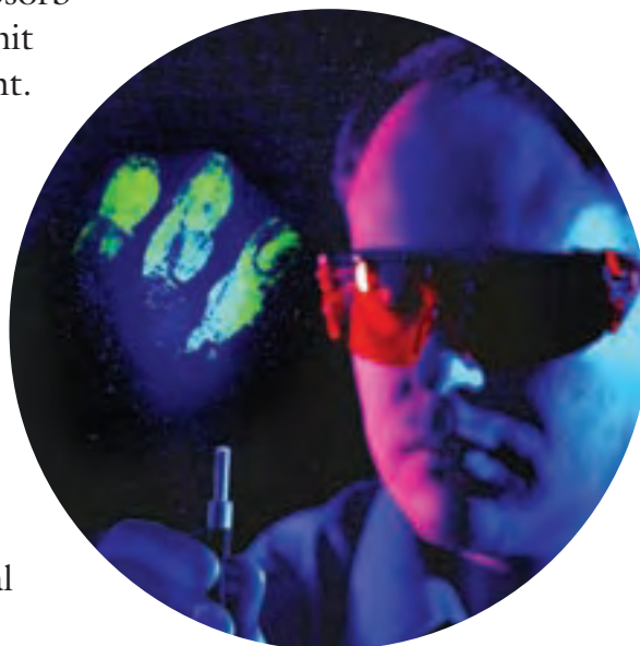
Figure 4.38 The detective is shining ultraviolet light on fingerprints dusted with fluorescent powder.
