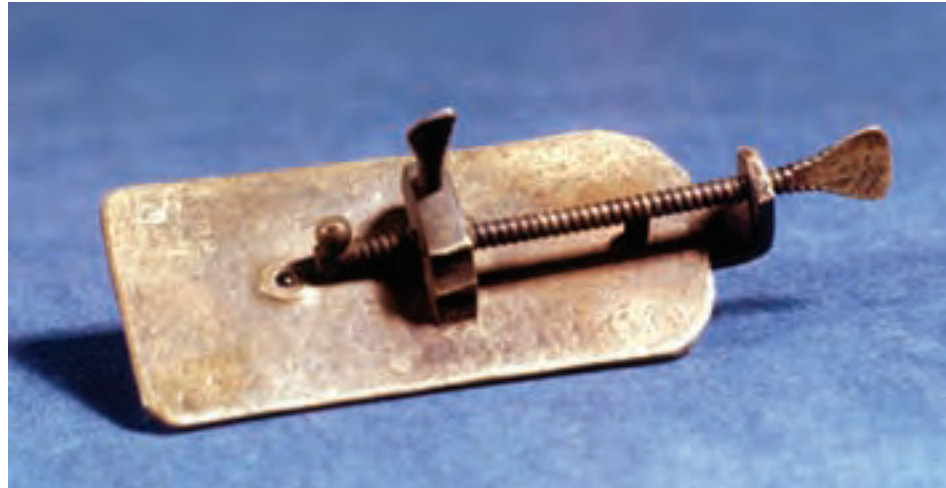
Figure 4.5 This probably does not look like a microscope but Leeuwenhoek discovered many “wee beasties” with it. The sample was placed on the point of the screw and Leeuwenhoek looked through a lens that was on the other side of the opening.
