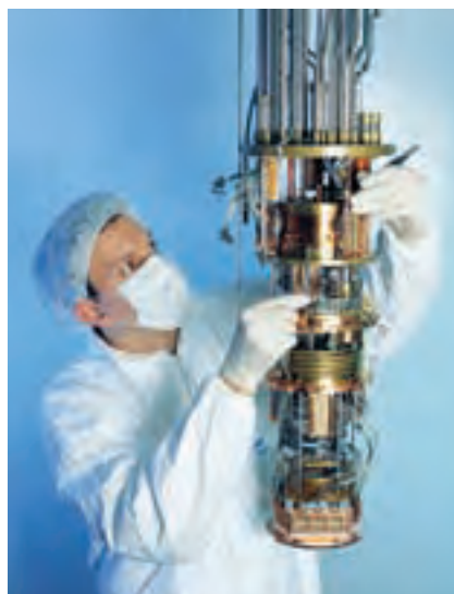
This device is a cryostat. A cryostat contains superfluid helium and is used to keep sensitive detectors at a stable low temperature.
