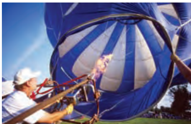
Figure 8.12 A hot-air balloon rises by adding heat to the air, and therefore decreasing the density of the air inside the balloon.
