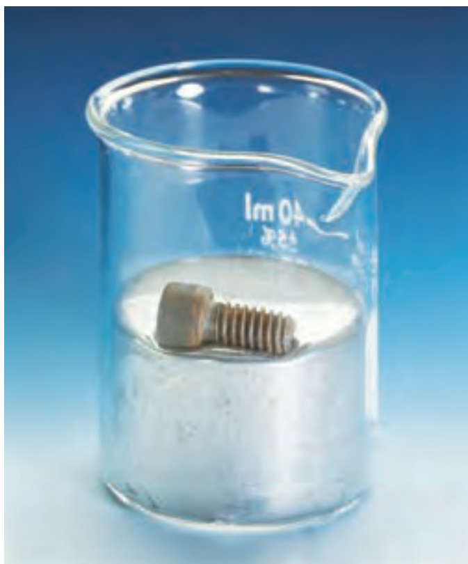
Figure 8.6A Liquid mercury is so dense that it can support a solid iron bolt. A layer of oil has been placed on top of the mercury to prevent vapour from escaping into the surrounding air, as mercury is very poisonous.
