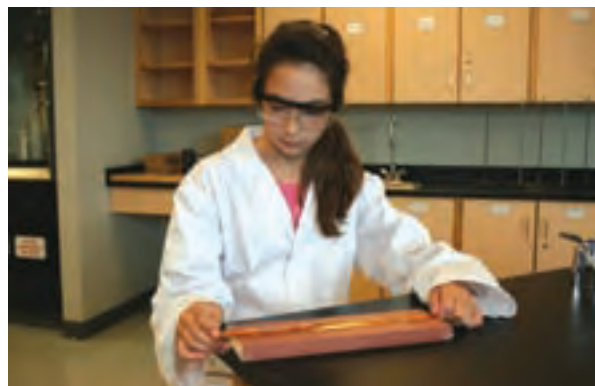
Figure 8.8 If an object has a regular shape, such as the block of wood in this picture, you can measure the length, width, and height and then use the mathematical formula, V = l \times w \times h , to calculate the object's volume.
