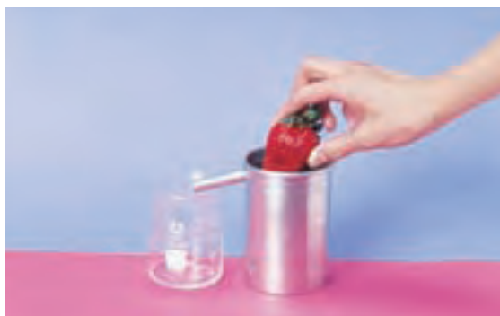
Figure 8.9 The volume of an irregularly shaped object can be found by measuring the volume of the water that spills out of an overflow can.
