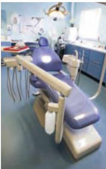
Figure 9.20 This dentist's chair uses hydraulic systems to adjust the height and position of the chair.
