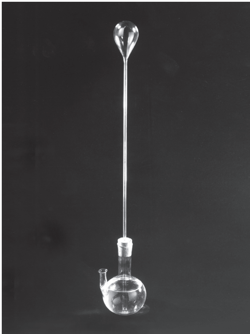
Figure 4.8 Galileo's original thermoscope looked much like this one. As the air warms, the coloured liquid drops down in the tube. As the air cools, the coloured liquid rises.
