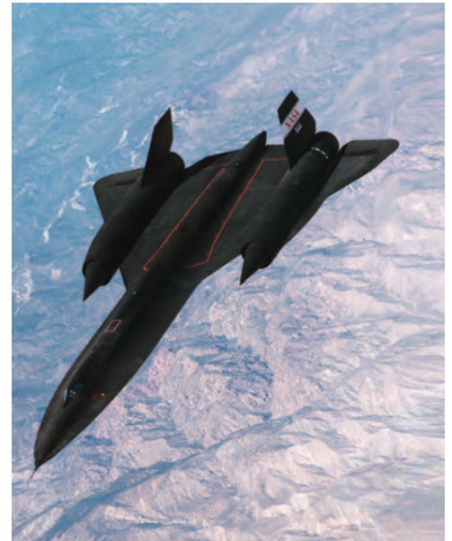
Figure 6.11 The SR-71 Blackbird has flown as fast as 3500 km/h. Although the black surface of the airplane radiates heat away as fast as possible, the surface gets so hot that the airplane expands several centimetres due to thermal expansion.
