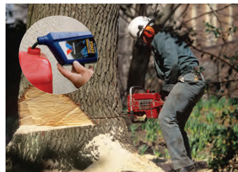
Figure 8.4 Small engines, like those in some lawnmowers and chainsaws, run on a solution of motor oil and gasoline. A certain volume of the oil is dissolved in a larger volume of gasoline. So, the oil is the solute and the gasoline is the solvent.
