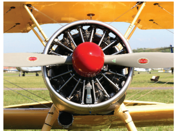
Figure 3.17 A propeller is made up of two or more twisted blades.
