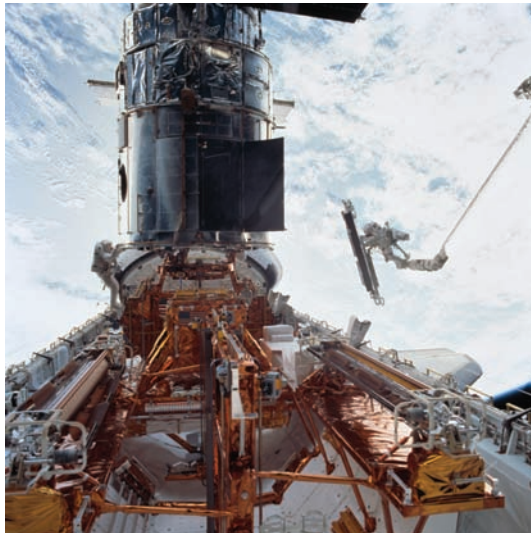
Figure 5.15 Look at the astronaut attached to the Canadarm. The astronaut is carrying an object toward the Hubble Space Telescope. The Canadarm also features the Canadian-developed and designed remote vision systems that allow the operators to see what they are doing.
