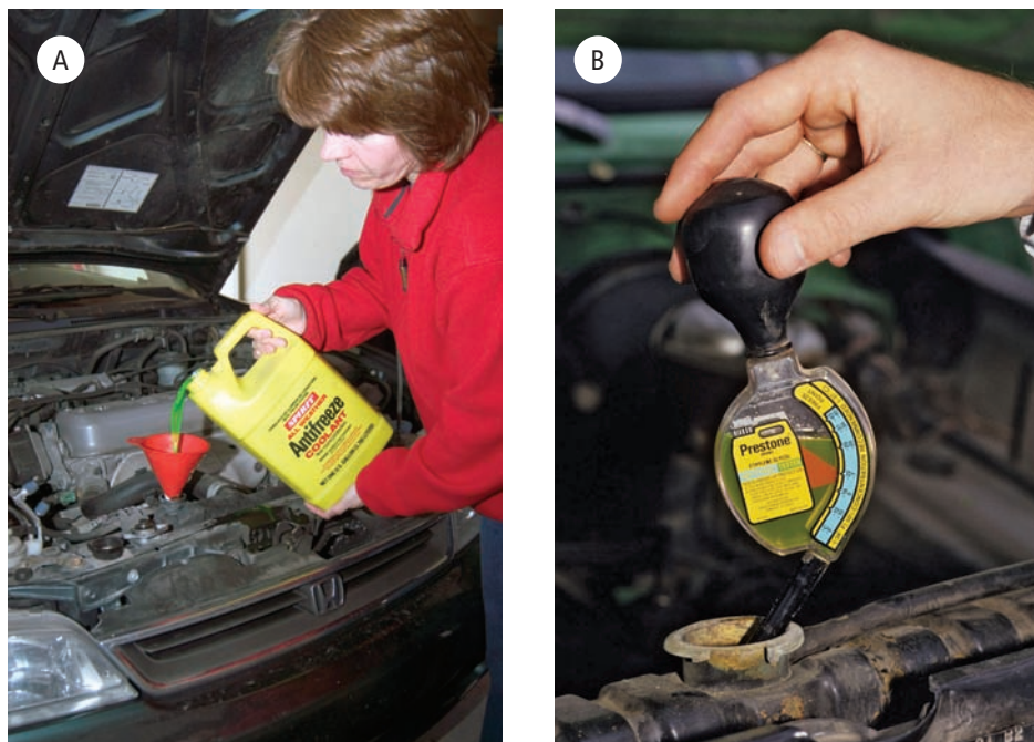
Figure 5.17 (A) The car owner is adding antifreeze to the car radiator. (B) To test the coolant, you squeeze the bulb then put the end into the coolant and release the bulb, drawing coolant into the tester. The dial will tell you the lowest temperature at which the coolant will still be liquid.
