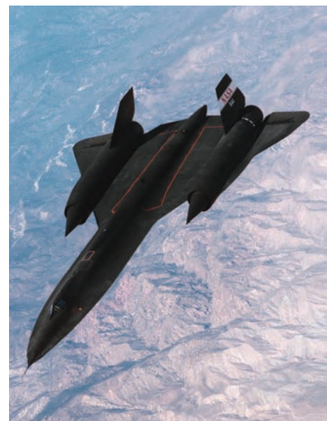
Figure 6.11 The SR-71 Blackbird has flown as fast as 3500 km/h. Although the black surface of the airplane radiates heat away as fast as possible, the surface gets so hot that the airplane expands several centimetres due to thermal expansion.
