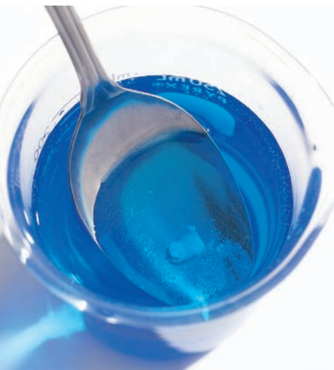
Figure 8.9 When 316 g of bluestone are dissolved in 1 L of water at 0°C, the bluestone solution is saturated. No more bluestone will dissolve in the solution at this temperature.
