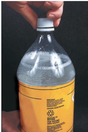
Figure 8.13 When the pressure of the carbon dioxide gas in a pop bottle decreases, the solubility of the gas in the liquid pop decreases. Bubbles of gas quickly come out of solution.
