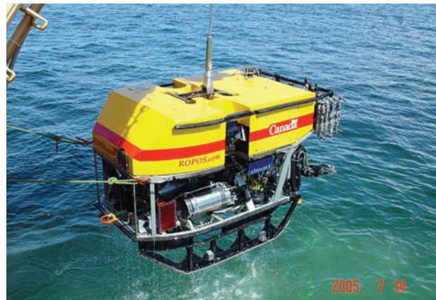
ROPOS is lowered into the ocean in a metal cage.
