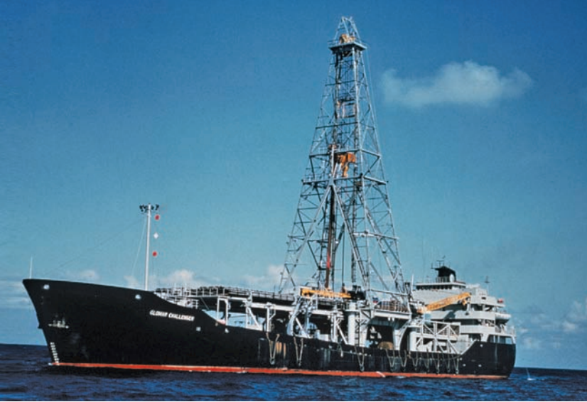
Figure 11.9 Scientists on the Glomar Challenger used oil drilling technology to sample the rock in one of the longest mountain ranges in the world, the Mid-Atlantic Ridge.
