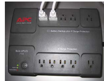
Figure 9.23 An electrical surge protector
