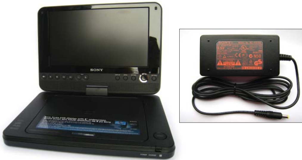
Figure 9.20 This portable DVD player has an adapter so that it can be plugged into a wall outlet or operated on battery power. This adapter supplies the device with a voltage of 9.5 V and a current of 2.0 A.
