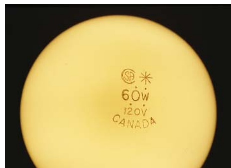
Figure 9.19 A 60 W light bulb converts 60 J of electrical energy into 60 J of light and heat every second.
