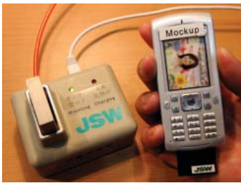
Figure 9.45 This micro hybrid hydrogen storage device, used to power a cell phone, is a prototype that was shown at the International Hydrogen and Fuel Cell Expo in Tokyo, Japan in 2007.
