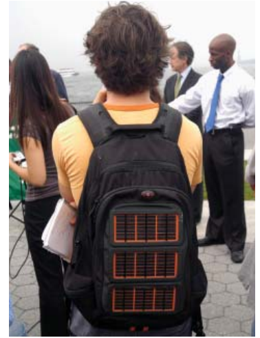
Figure 9.43 Solar bags contain solar cells designed to charge the batteries in laptops, cell phones, and MP3 players.
