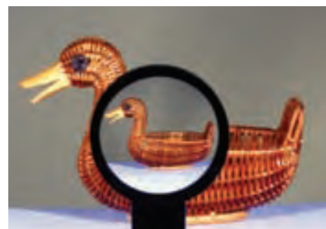
Figure 6.12 A concave lens never produces an image that is as large as or larger than the object.
