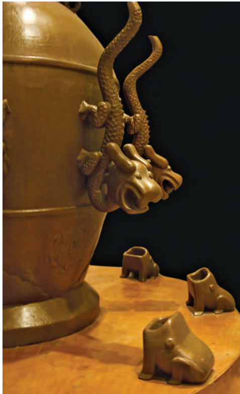
Figure 11.15 An ancient earthquake detector from China. The eight dragons on this urn have little balls inside them. Earthquake movements shake the balls into the toads' open mouths. The direction of the earthquake is determined by which toad swallows the ball.
