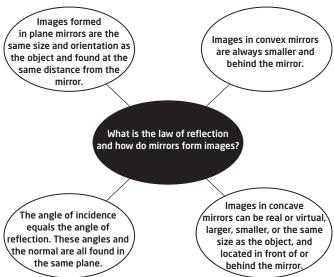
**2.** The angle of the incident ray is equal to the angle of the reflected ray, the incident ray and reflected ray are on opposite sides of the normal, and both rays and the normal are on the same surface or plane.
