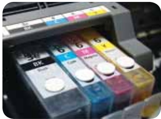
▲ Figure 4.15 Most printers use only three pigment colours as well as black.
