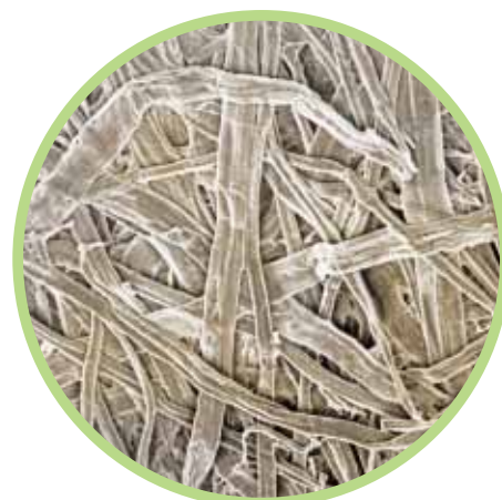
▲ Figure 4.19 When you look at paper under a microscope, you see that the surface is actually very rough.
