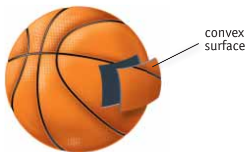
▲ Figure 4.31 If you cut a section from a basketball and cover the outside surface with a reflective material, you would have a convex mirror.
