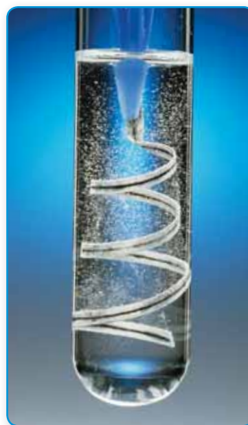
Magnesium reacts with aqueous hydrochloric acid.
