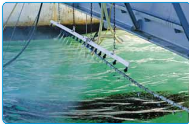
Figure 4.24 A chemical is being applied to an oil spill test tank to determine how efficient it is in breaking up the oil.
