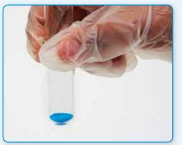
You only need to add enough of the copper(II) sulfate, shown here, and the other solids to fill the rounded bottom of each test tube.
