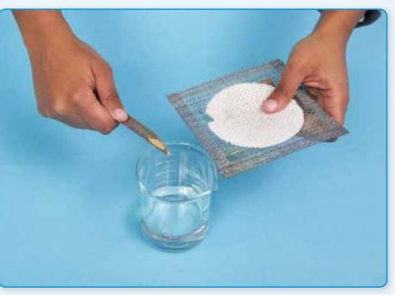
Cover the beaker with a wire gauze pad immediately after adding yeast to the hydrogen peroxide.
