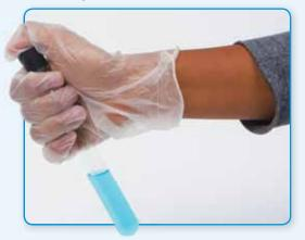
To shake the test tube safely, hold it as shown. Gentle shaking is all that is needed.
