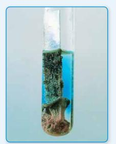
Zinc metal in an aqueous solution of copper(II) sulfate will undergo a reaction.
