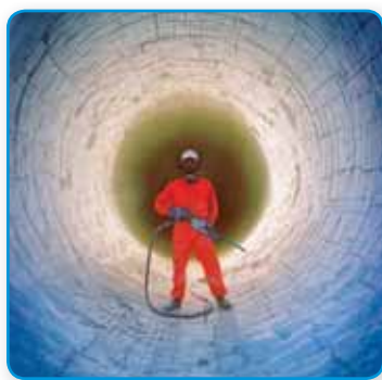
Figure 5.10 This worker is standing inside a kiln that is used for heating calcium carbonate. Kilns are ovens used for heating or drying materials.
