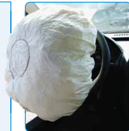
Figure 5.9 Airbag technology has relied on the decomposition of sodium azide. The reaction is triggered by an electrical impulse, and nitrogen gas is produced, which inflates the bag.
