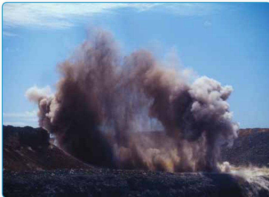
Figure 5.8 Explosives, like the ones used in this coal mine blast, produce tremendous force to break apart rocks. They can occur as a result of the decomposition of a compound and the rapid heating and expansion of the gases that are produced.
