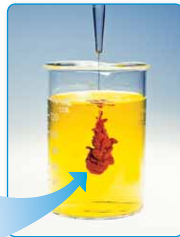
Figure 5.16 A red precipitate, \text{Ag}_2\text{CrO}_4(\text{s}) , forms when two ionic solutions, \text{AgNO}_3(\text{aq}) and \text{K}_2\text{CrO}_4(\text{aq}) , undergo a double displacement reaction.
