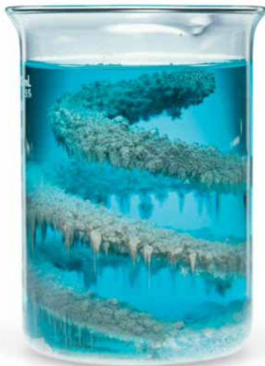
Figure 5.12 In the single displacement reaction between copper metal and aqueous silver nitrate, copper displaces the silver to produce a blue copper(II) nitrate solution and solid silver deposits.
