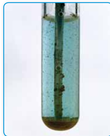
Figure 5.15 As magnesium metal reacts with an aqueous solution of copper(II) sulfate, copper metal forms.
