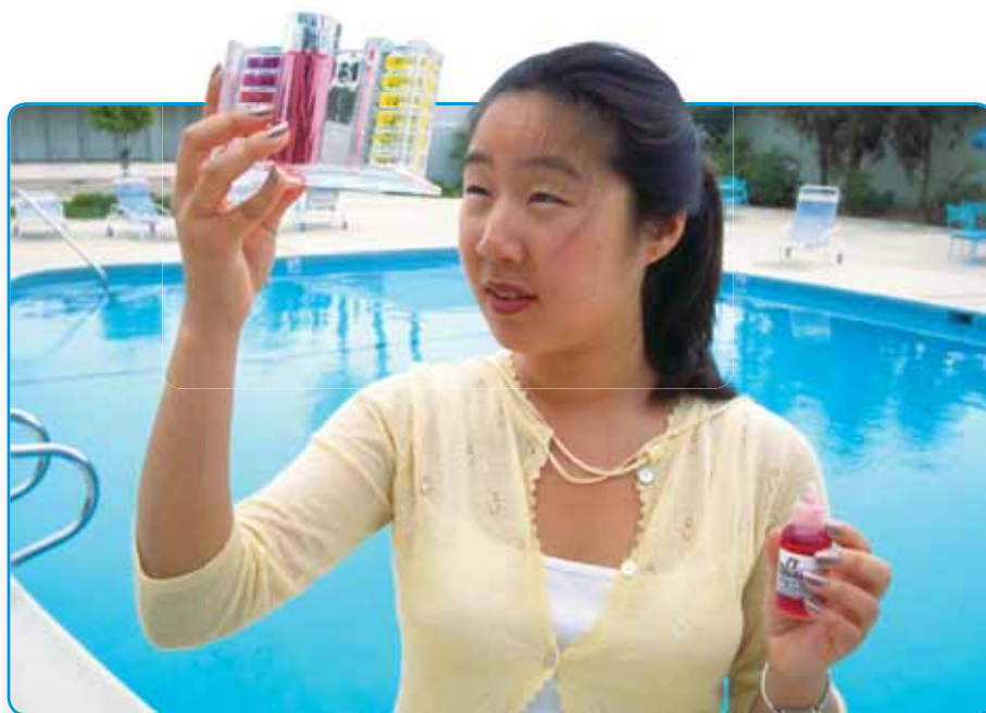
Figure 5.23 An understanding of pool chemistry is needed to monitor the levels of chlorine-based chemicals. These chemicals are used to keep pools clean and free of algae and bacteria.
