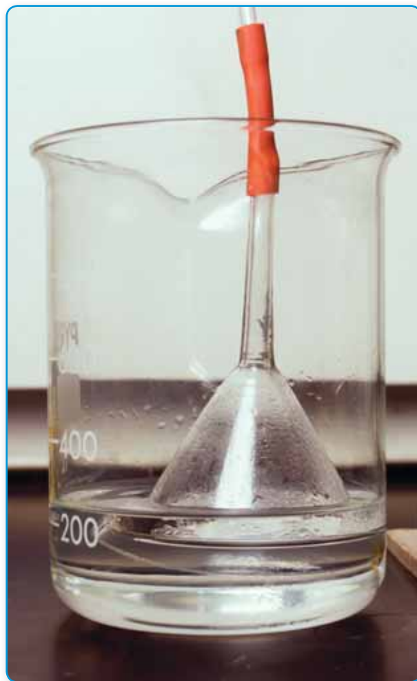
Figure 6.2 Hydrochloric acid, \text{HCl}(\text{aq}) , forms when hydrogen chloride gas, \text{HCl}(\text{g}) , is added to water. The resulting solution contains hydrogen ions and chloride ions.
