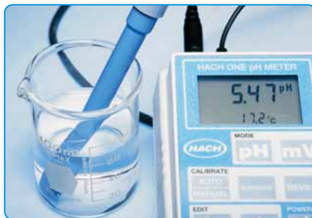
Figure 6.9 The pH meter shows that this solution has a pH of 5.47 and is acidic.
