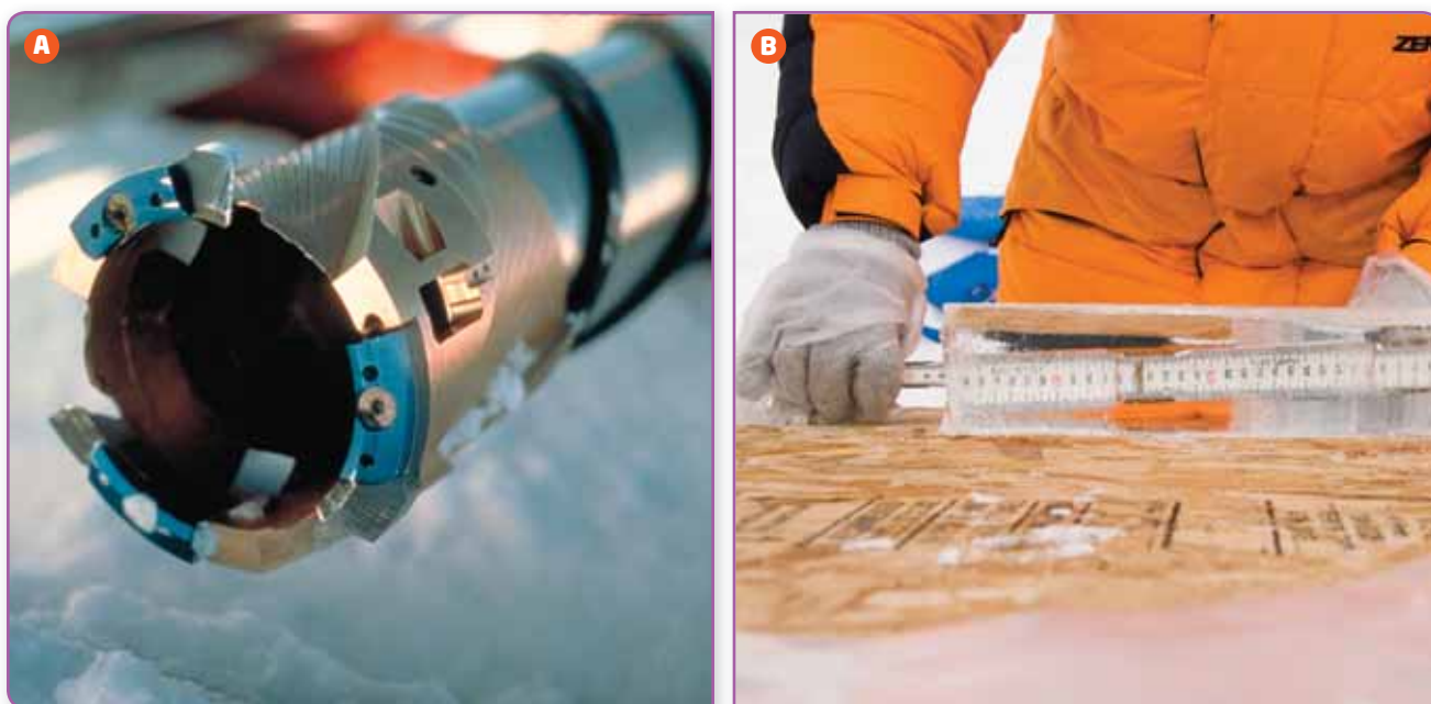
Figure 9.2 Scientists use A a special drill to obtain B ice cores. A drill can penetrate to a depth of 50 to 70 m in one day. This depth is equivalent to about 200 years of ice build-up.
