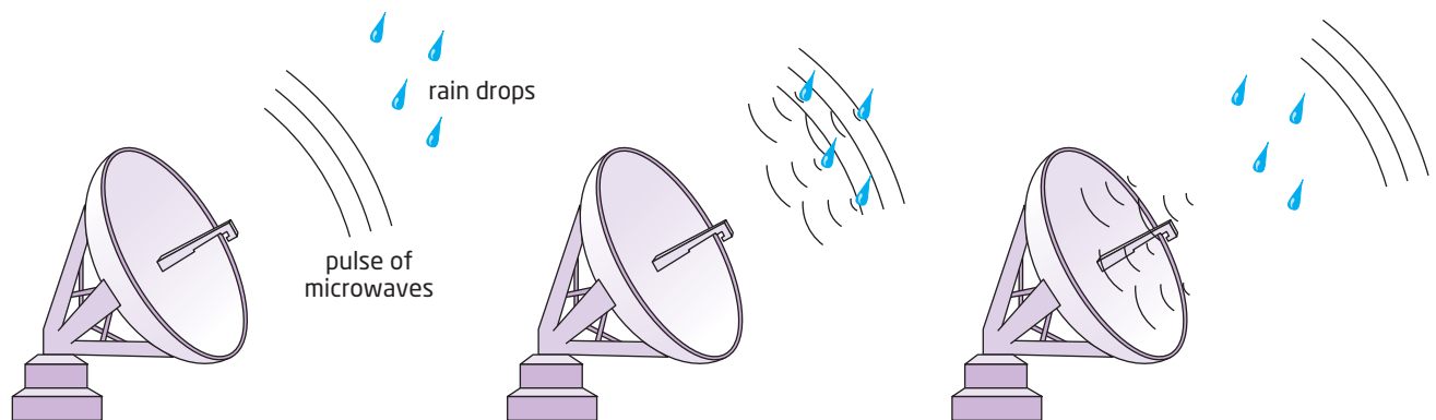
Figure 9.10 A radar instrument transmits short pulses of microwaves that move through the air until they strike an object, such as a raindrop or a snowflake. The object reflects some of the waves back to the radar instrument, thus communicating information about conditions in the atmosphere..
