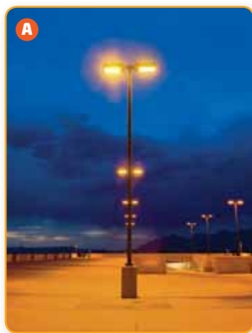
Figure 10.3 A The yellow light that is emitted by many streetlights is produced by excited sodium atoms. B Electric charges move rapidly between the electrodes, colliding with the atoms in the vapour and exciting them.
