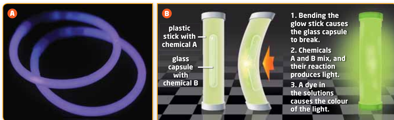
Figure 10.8 A You have probably seen many of these glow sticks in the form of bracelets or necklaces. B When chemicals A and B mix, the reaction produces light.
