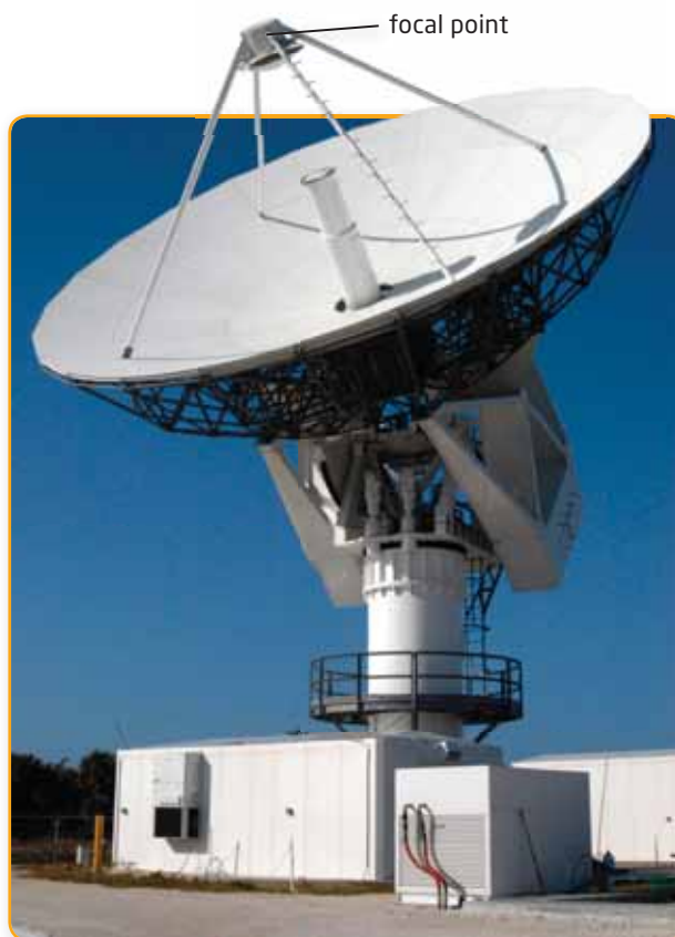
Figure 10.23 A radar antenna acts as a concave mirror for radio waves.
