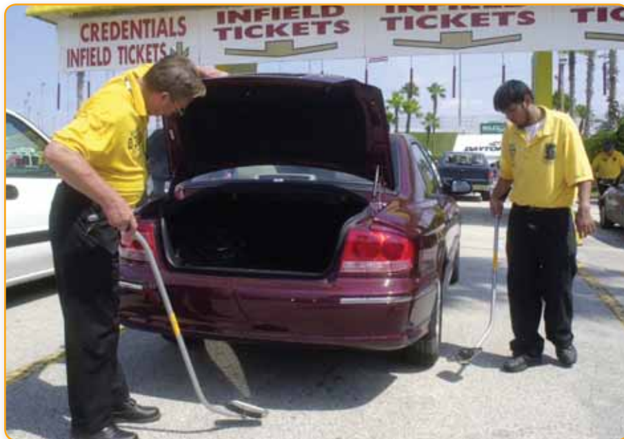
Figure 10.28 Using a convex mirror on a long handle enables a security guard to see the underside of a vehicle without crawling under it.
