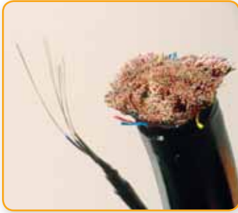
Figure 11.21 The small optical fibres can carry as much information as the large copper cable on the right.
