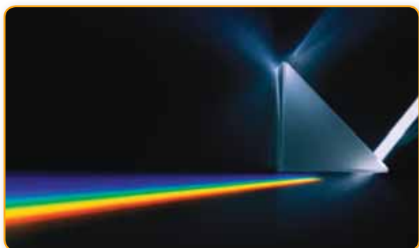
White light entering a prism is partially reflected and refracted.
