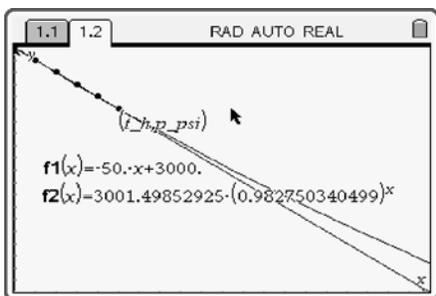
With the  $y$ -axis set to display from 2000 psi to 3000 psi, the graphs start to show a visible difference after approximately 7 h.
