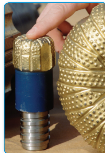
Figure 4.13 Diamonds have been embedded into the ends of these drill bits to make it easier for the drills to cut through rock.
