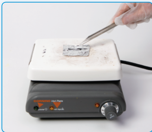
Place each substance on a piece of aluminum foil that is placed on the hot plate.
