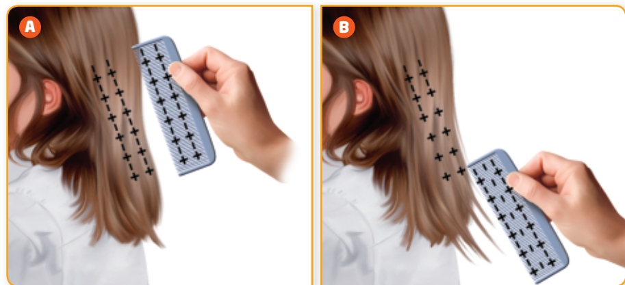
Figure 10.3 Look carefully at the + and – symbols. A Before combing, both the girl's hair and the plastic comb are neutral. B After combing, the girl's hair is positively charged, and the comb is negatively charged.
