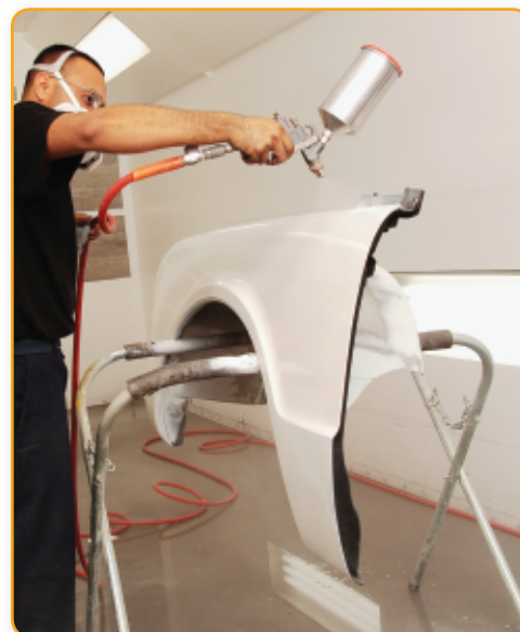
Figure 10.21 Electrostatic spray painting is a good environmental and economic choice because it reduces over-spraying.
