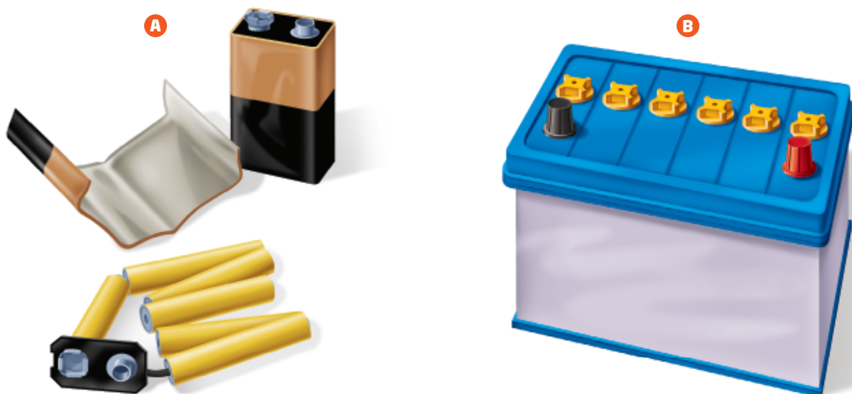
Figure 11.23 A The familiar 9 V battery contains six 1.5 V cells connected together. B An automobile battery contains six 2 V cells.
