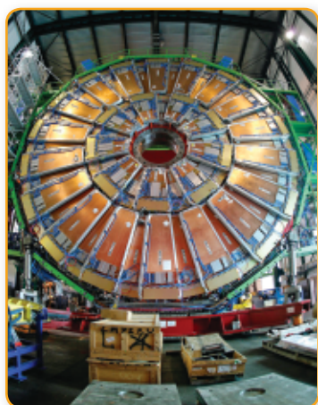
Figure 11.26 The enormous magnet in the Large Hadron Collider at the European Centre for Nuclear Research (CERN) is the largest superconducting magnet ever built. It uses a current of 21 000 A, but it has a potential difference of only about 9 V.
