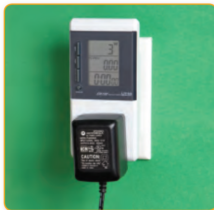
Figure 12.15 You can measure the power that an appliance uses by connecting it to a watt-meter. You can also use the meter to measure the phantom load (if there is one) when an appliance is turned off.
