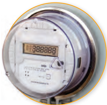
Figure 12.12 Smart meters encourage conservation by making us think about how and when we use electrical energy.
