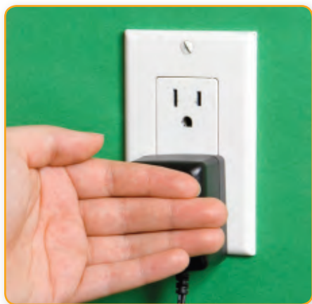
Figure 12.14 External power adapters are sometimes called wall warts. These adapters are inefficient and give off a substantial amount of heat.
