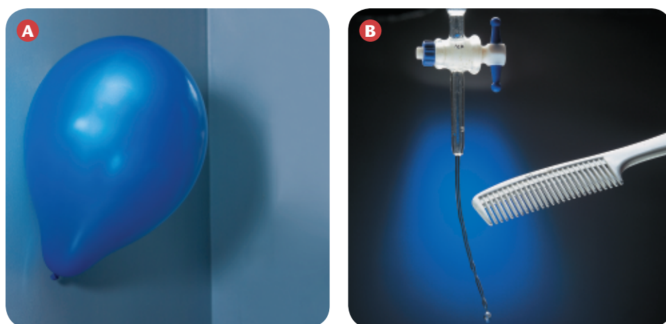
◀ Figure 4.6 The balloon in photo A is charged, but the wall is not. The comb in photo B is charged, but the water is not.
