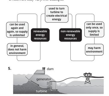
Water flows through the dam, which causes a giant turbine to spin. This causes the generator to create electrical energy. The energy is then sent through wires for home use and and other uses.
