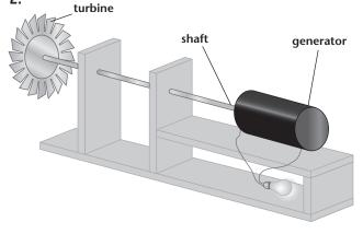
A generator system works as follows: Some energy source is used to turn the turbine. The turbine causes the shaft to rotate, which creates kinetic energy. The generator transforms this kinetic energy into electrical energy.
